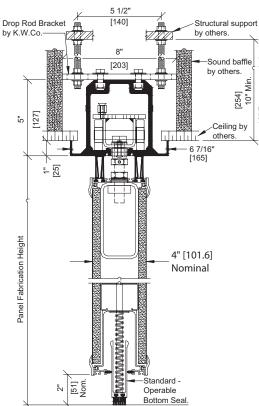
H.D. Curve & Diverter Steel Track and Carrier
