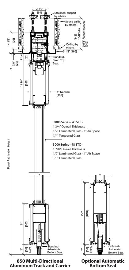
2 1/2" Structural support by others. Sound baffle 8 3/8" Recommended [213] by others. 2 7/8" 3/4" [121] 7 Optional-Operable Top Seal 7/8" [22] 11 1/4" [286] 4" Nominal [102] Panel Fabrication Height 7 1/2" [191] [610] 2'-0" 1'-0 3/4" [202] Optional -[51] Nom 5 . Operable Bottom Seal.
