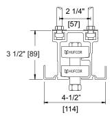
Type 26 Aluminum Track Optional for panel weights to 500 lbs. [227 kg]. Each carrier has two horizontal counter-rotating wheels. Each wheel has precision ground bearings, encased with Delrin for quiet operation. Minimum dimension from the ceiling to the structure is 8" [203].
