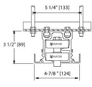
**Type 36 Aluminum track**. Standard for weights to 1000 lbs. [455 kg]. Shown with optional suspension bracket available for 5-1/4" [133] spacing. Suspension bracket is available for all aluminum tracks.
