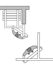
Top Supported Side Stack Individual, Omni-Directional Panels Manually Operated Maximum Height: up 41'7" [12.5m] \* Maximum Opening Width: Unlimited STC Ratings: 52, 54, 56
