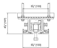
Type 11L Steel Track For panel weights to 1400 lbs. [635 kg]. Track is of 3/16" [5] formed steel. Track trim is clear anodized aluminum. Each carrier has four steel wheels with precision ground radial bearings. Minimum dimension from the ceiling to the structure is 8" [203].
