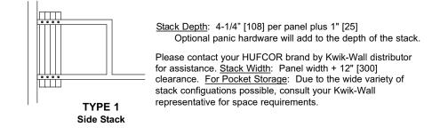
The Type 1 stack shown above is the most often used for simple omni-directional layouts. Following are additional common stack configurations. Stacks are not limited to these configurations and may be built to fit each job requirement. Consult your representative for design assistance.
