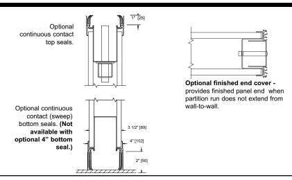
**OPTIONAL TRACKS** - Alternate track systems may be used providing the height and weight limits are within manufacturer's guidelines.
