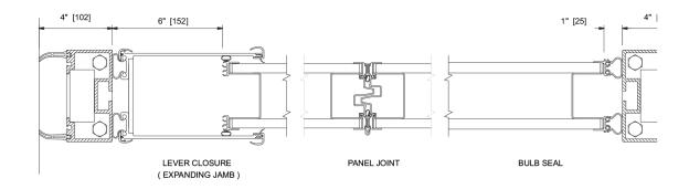
Stack Size: To determine the stack depth, refer to the specifications for the operable partition model used in the Unispan. Remember to add 4" [102] for the support column (a/k/a post).
