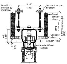
850 Hinged Pairs Steel Track and Carrier
