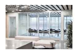
**LUNA** – at a sleek 2-3/4" aluminum panel frame thickness, Luna sliding and folding glass partitions combine designer aesthetics with 43 STC high-performance sound control.
